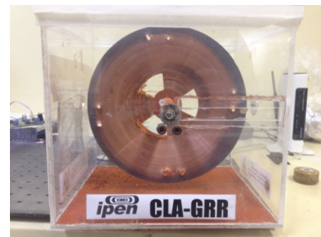
Figure 12. Laser decontaminated plate from a radioactive lightning rod. The thin powder at the bottom contains the contaminant and can be easily stored; the plate can then be recycled.
